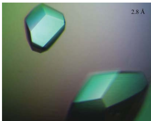
Figure 11 Crystals of a heat-treated viral protein–ligand complex diffract to 2.8 \text{\AA} . The addition of 0.1% \beta -octylglucoside to the protein solution was required to grow crystals of some of these complexes.
